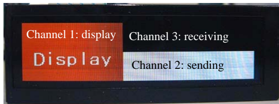
Fig. 4 Panel division for multiple channel access.
