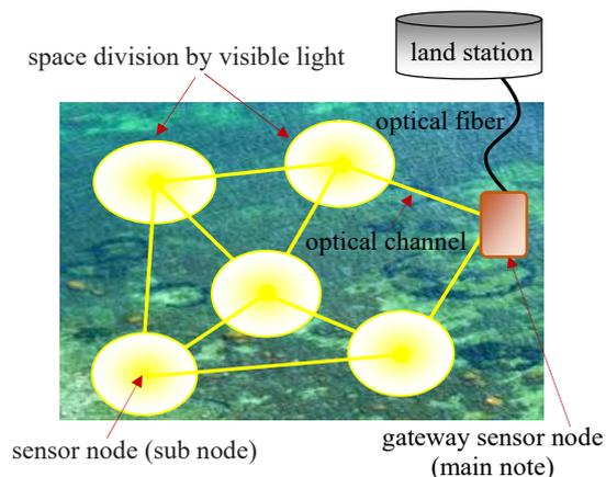
Fig2. The underwater optical wireless sensor network.
