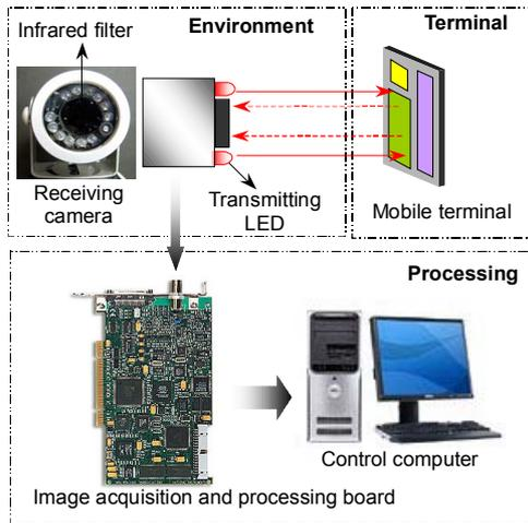
Fig. 2 The optical wireless communication system.
