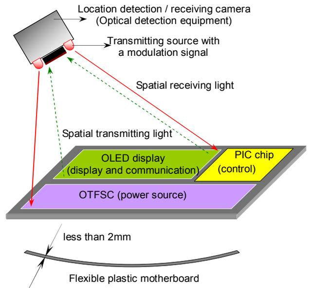
Fig. 1 The terminal structure and its work method.
