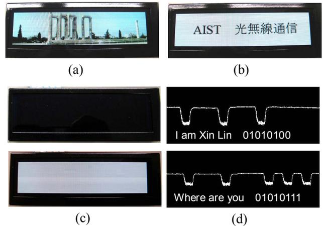
Fig. 4 Examples of display and communication using the OLED module: (a) displaying an image, (b) displaying letters and characters, (c) The transient image for code "0" and "1", and (d) transmitted signals.
